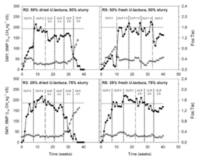
Specific methane yield, BMP and organic acid to alkalinity ratio (Fos:Tac) from continuous operation with different mixtures of dried and fresh seaweed (*U. lactuca*) and dairy slurry (Allen et al., 2014).
