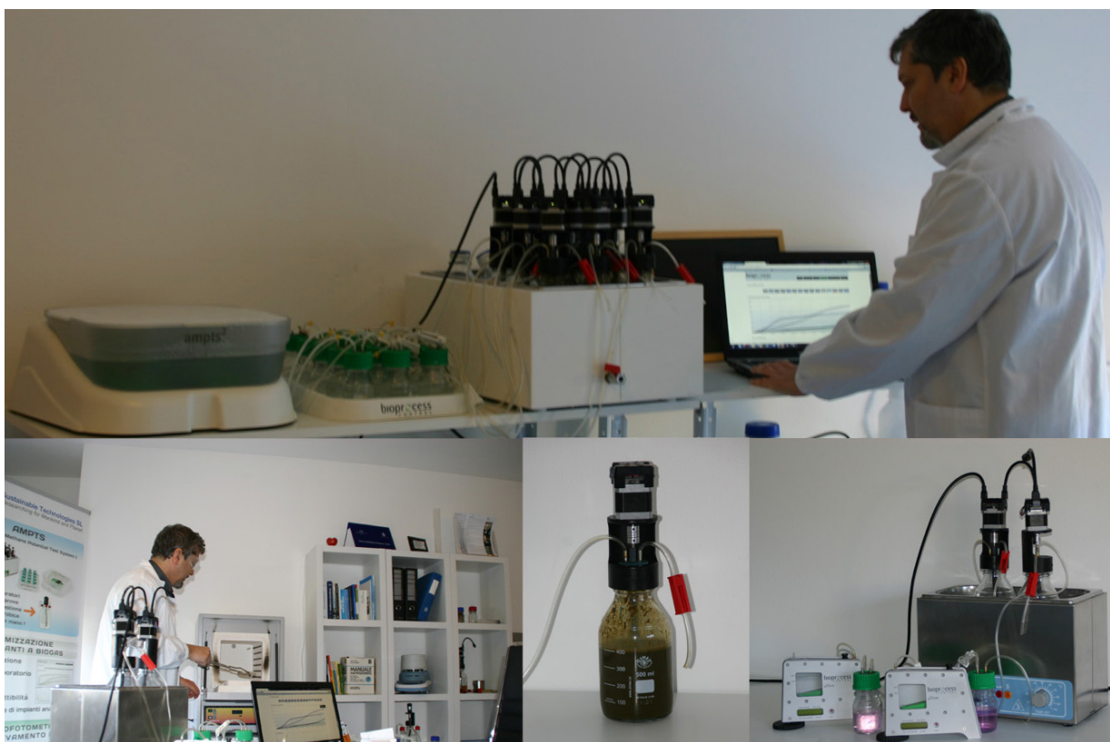
Figure 1: Example of field laboratory to measure the BMP of silage and other substrates
