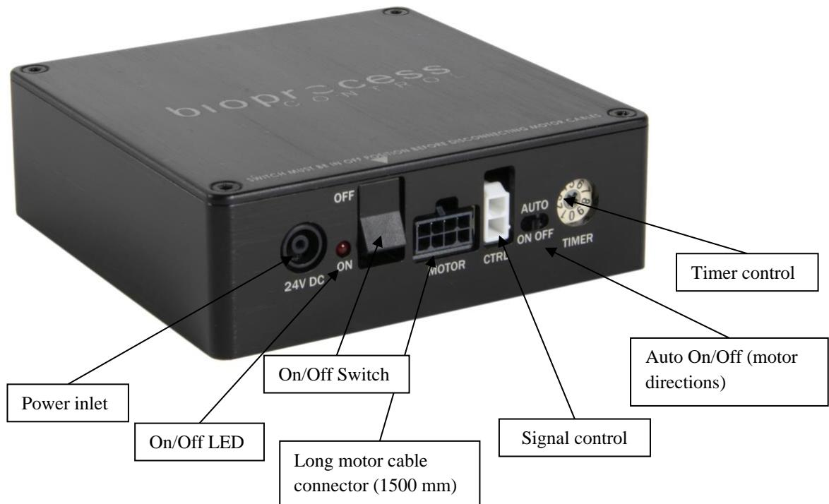
The **ON/OFF switch** (shown in the picture above) controls the power of the Motor Controller. When the switch is ON, the red LED will be lit in order to indicate that the system is active. It is required to set the switch to OFF before connecting / disconnecting the Motor Controller to / from the power mains.
