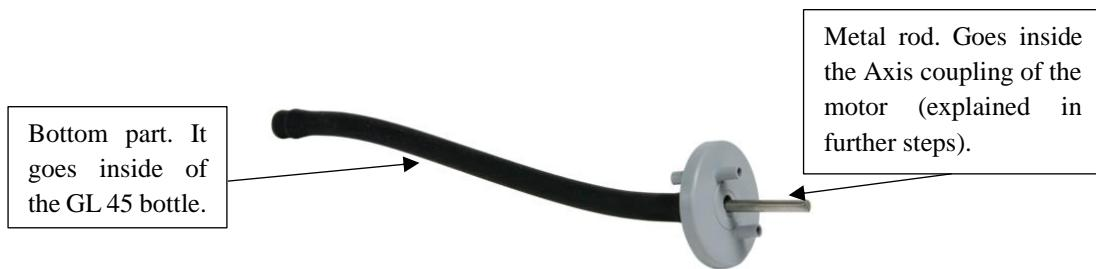
The metal rod has two bending points, they divide the bending rod into 3 parts (one short end, one long end and the middle part). The shorter end should always go inside the rubber part of the stirrer, the longer part should be directed towards the Axis coupling.
